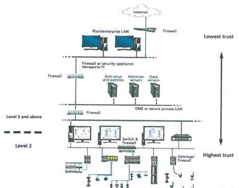
Components that are not as critical to safety and availability, such as historians and data servers, should be installed at an upper level in the hierarchy, with less protection, but correspondingly more access, so that plant personnel can view data and make changes as needed.
