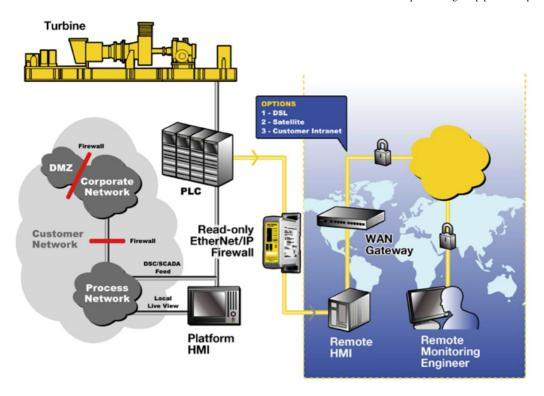
This system example shows the deployment of an EtherNet/IP read-only controller firewall in a natural gas turbine protection system.
