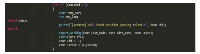
Figure 14: Reporting details of successfully breached devices.
