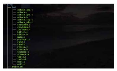
Figure 10: Different modules of the Mirai bot.
