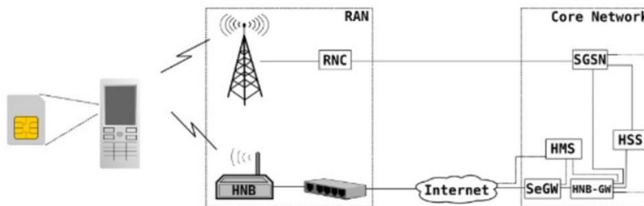
Figure 6. Femtocell connection map
