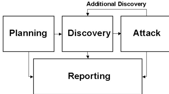
**Figure 3.1 - Four-Stage Penetration Testing Methodology**
