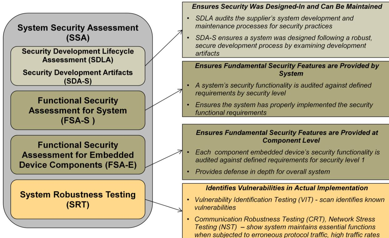
**Figure 1 - Evaluation Elements for ISASecure SSA Certification**
