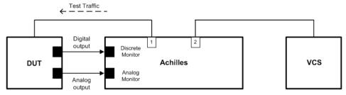
Both digital and analog outputs are monitored by the Achilles®:
