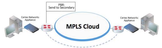
**Test Results:** Although the data was encrypted, the traffic successfully bypassed the MPLS network based on the PBR port based rule. The CE router had no problem applying PBR rules based on the Layer 4 information of packets encrypted by CipherEngine.
