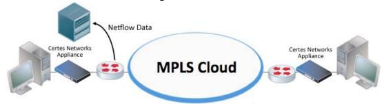
**Test Results:** The Netflow analyzer successfully collected address, protocol and port information after the data was encrypted using Layer 4 encryption.
