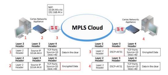
**Test Results:** Even though the address translation occurred after encryption, Certes Networks was able to successfully decrypt the NAT'd packets. Traffic was properly decrypted at the other end with the NAT'ed IP address on the clear packet after decryption.
