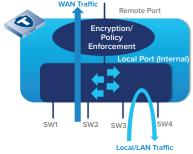
The diagram to the left illustrates how WAN traffic is passed through the switch and to the policy enforcement engine, while LAN traffic is switched locally, so it doesn't use any CPU cycles.
