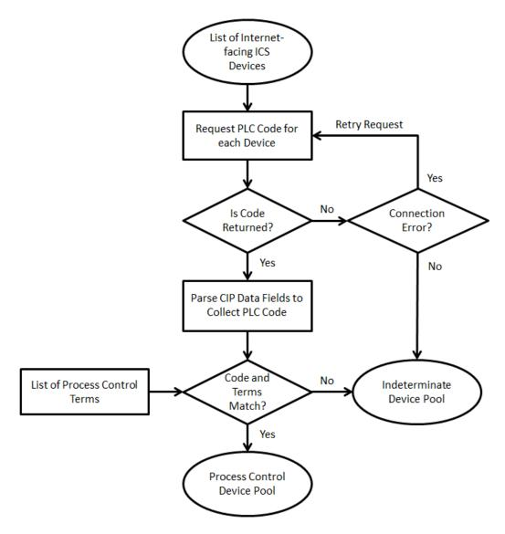
Figure 3.1: Process to Distinguish Internet-facing ICS Devices.
