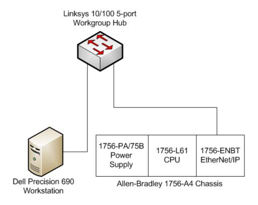
Figure 4.1: Hardware configuration for exploratory testing.
