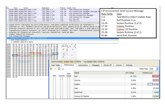
Figure 3.6: Task Monitor Graphical Interface shown with Wireshark CIP packet capture.
