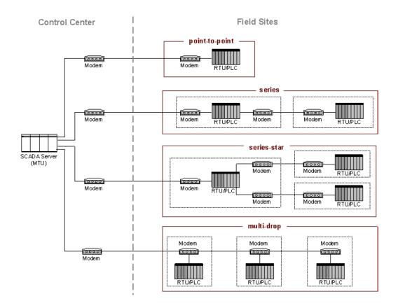
Figure 2.3: NIST SCADA Communication Topologies [20].
