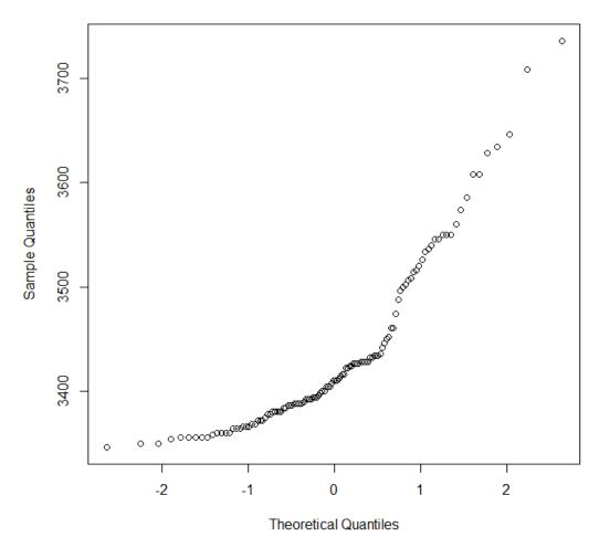
Figure 4.7: R Q-Q Plot of PLC Task Execution Times L61 v16.56.47.
