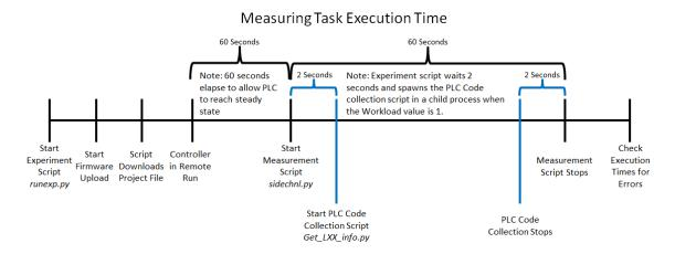
Figure 3.7: Measuring PLC Task Execution Times.
