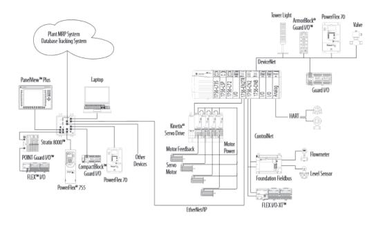
Figure 2.5: Allen-Bradley ControlLogix PLC Architecture [25].
