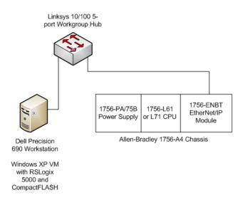
Figure 3.4: ControlLogix Experiment Architecture.
