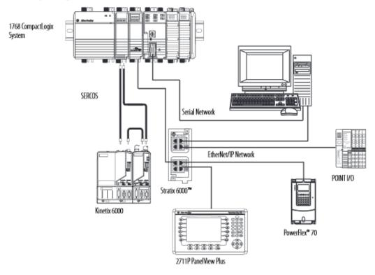
Figure 2.8: Allen-Bradley CompactLogix PLC Architecture [27].
