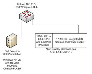
Figure 3.5: CompactLogix Experiment Architecture.
