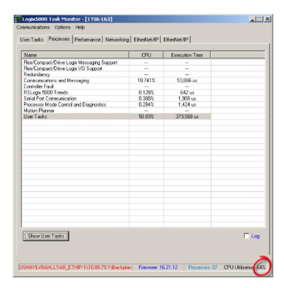
Figure 2.9: RSLogix Task Monitor.
