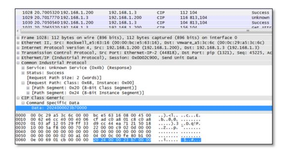
Figure 4.3: PLC Code Request for Global Instance Values.
