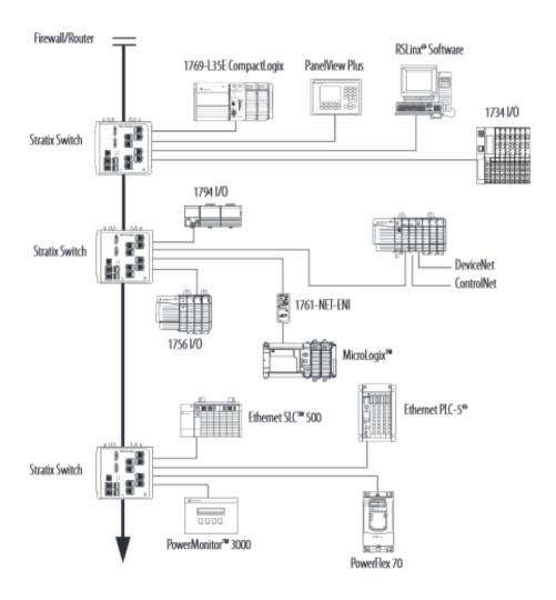
Figure 2.6: Allen-Bradley EtherNet/IP Architecture [25].
