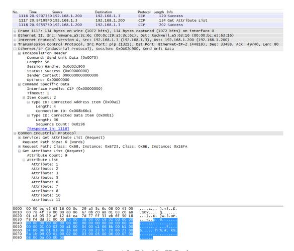
Figure 4.2: EtherNet/IP Packet.
