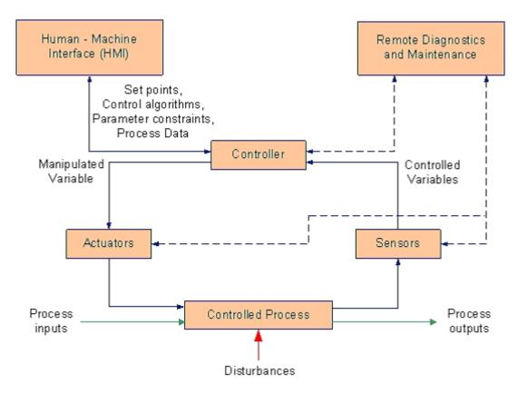
Figure 2.1: ICS Operation Function Blocks [20].
