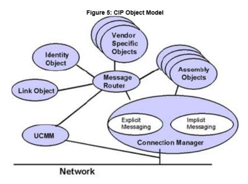
Figure 2.13: Common Industrial Protocol Object Model [6].
