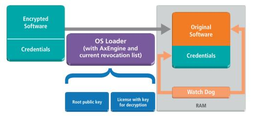
Figure 4: Integrity verification (Forward-Check)
