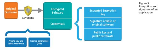
The verification consists of the following steps, which are executed while the application is being loaded. This is performed with the aid of a system integrated tool, the AxEngine from WIBU-SYSTEMS.
