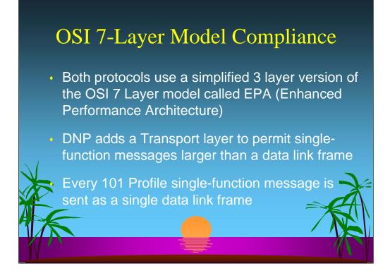
In DNP all application layer functions are implemented as application layer messages encapsulated in data link frames.
