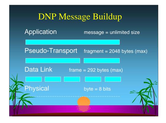
•Receive goes up the stack, transmit goes down the stack.
