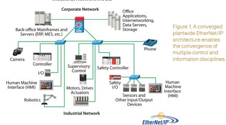
To design and plan a plantwide EtherNet/IP network, first consider each level of the logical model shown in Figure 2. Then generate a network requirements document using industry best practices and standards. Be sure to include any required future expansion capabilities.
