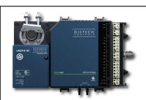
1A-VAV: VAV box controller with multiple analog inputs and outputs. Also incorporates dedicated actuator and pressure sensor (normally Tier 0 devices). Network is LonTalk over TP/FT-10 media at 78 Kbps.
