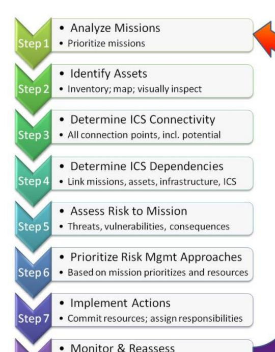
Figure 1. ICS Security Assessment Eight-Step Process
