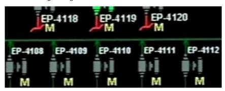
Figure 8: Very different valves: While the stage exhaust valves (labeled EP-4108 to 4112 in this partial screenshot from the CPS SCADA display) stay closed during normal operation *and during the attack*, at least one of the feed valves (labeled EP-4118 to EP-4120) must stay open. Pressure controllers at the product and tails take-offs must also be compromised to not signal a low pressure condition.
