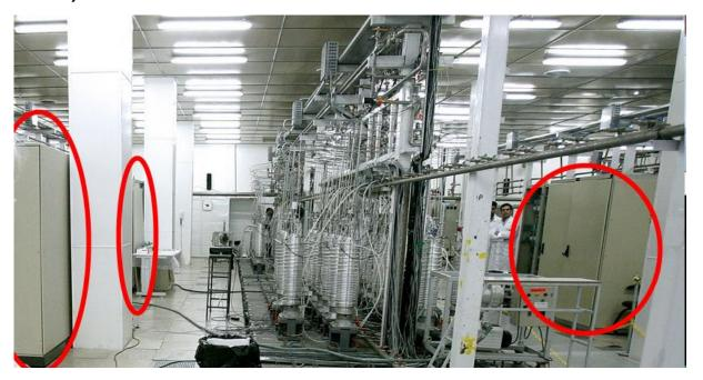
Location of control system cabinets in the above-ground Pilot Fuel Enrichment Plant (PFEP). Although it cannot be seen in the picture, the Siemens S7-417 and S7-315 controllers compromised in the attack are almost definitely located inside these cabinets — which will likely have been accessed directly by the control system engineers who unwittingly infected the controllers with Stuxnet.
