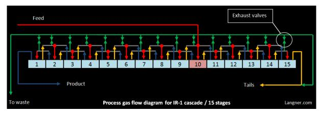
In this diagram, standard I&ID valve symbols are used for stage exhaust valves. Symbols show all exhaust valves open, as would be the case during contingency dump of the whole cascade.
