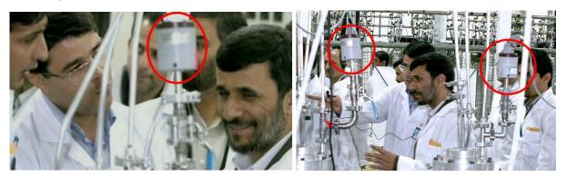
Various pictures show the pressure sensors used in Natanz. On the SCADA screens they are labeled with "PT-", which obviously stands for "Pressure Transducer". According to our intelligence, Iran uses MKS Baratron sensors, maybe also MKS clones. The following shows an MKS Baratron transducer as photographed by the manufacturer.
