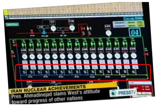
The key is the piping *below* the fifteen enrichment stages, highlighted in red. It is equipped with valves that would allow to simply "valve off" leading and trailing stages in order to arrive at a reduced cascade shape with less than fifteen stages. Any other reason for the valves other than to modify the number of enrichment stages is not evident.
