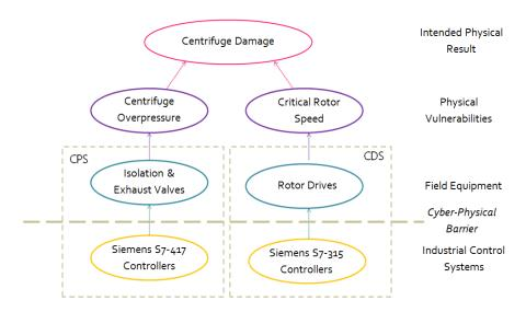
Figure 2: Synopsis of the two different attacks implemented in Stuxnet. Both use a manipulation of industrial control systems to achieve physical damage, exploiting different physical vulnerabilities of the equipment (centrifuge rotors) that basically lead to the same physical result
