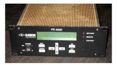
The pressure controllers must be compromised in order to disable the Cascade Protection System's stage exhaust valves. This suggests a link between the Cascade Protection System's main controller, the Siemens S7-417, to the pressure controllers. Since the PR-4000 doesn't come with a built-in PROFIBUS interface, communication is most likely established via a PROFIBUS-to-serial gateway, as shown in the diagram below; a configuration that is used in similar
