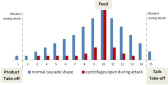
Figure 6: Modified cascade shape during the attack. Isolating all centrifuges in stage 1 and 15 effectively blocks the outflow of process gas, resulting in an increase in pressure for the non-isolated centrifuges
