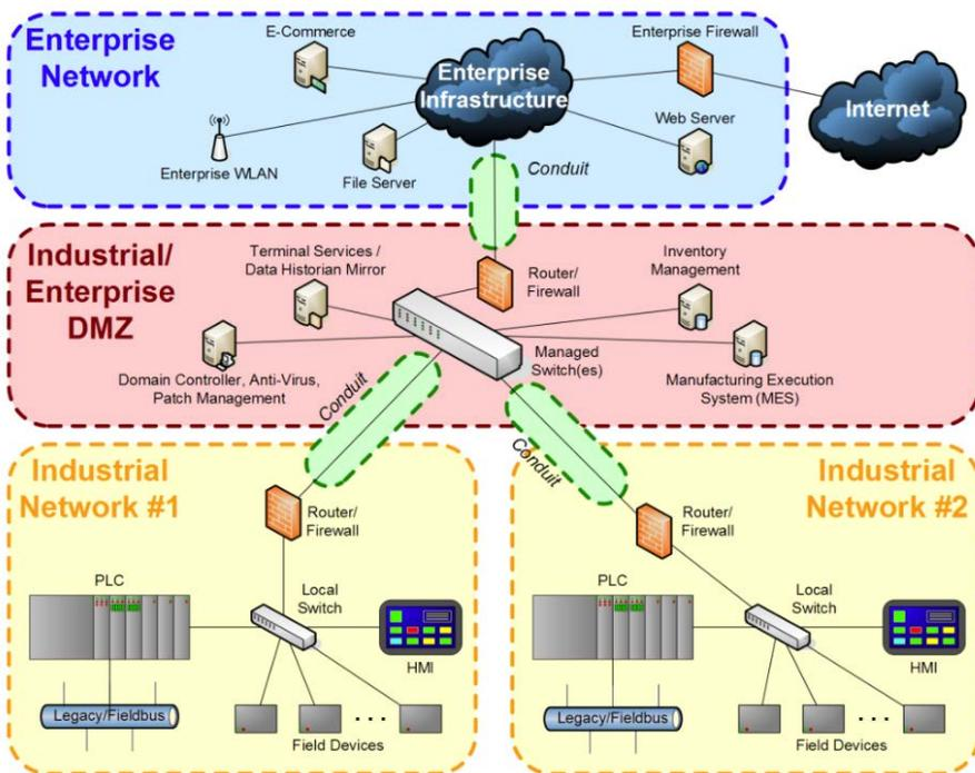
Figure 8: ICS Reference Architecture – Zones and Conduits (source: isa.org)
