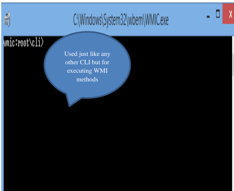
Figure A-3: Administrators and malicious attackers can use the Wmic.exe terminal to execute WMI methods.
