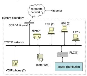
Figure 2. Simplified network diagram of Case Study 2 (SCADA).
