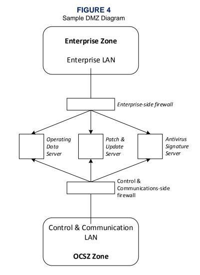
A separate authentication server may be employed with the DMZ so as to validate employee remote or vendor connections coming through the Enterprise Zone to the OCSZ. VPN connections using IPSec or SSL are frequently included in the firewall internals in today's products on the market.
