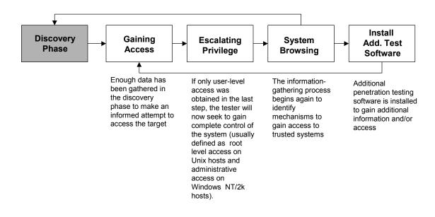
Figure 3.2 - Attack Phase Steps with Loopback to Discovery Phase
